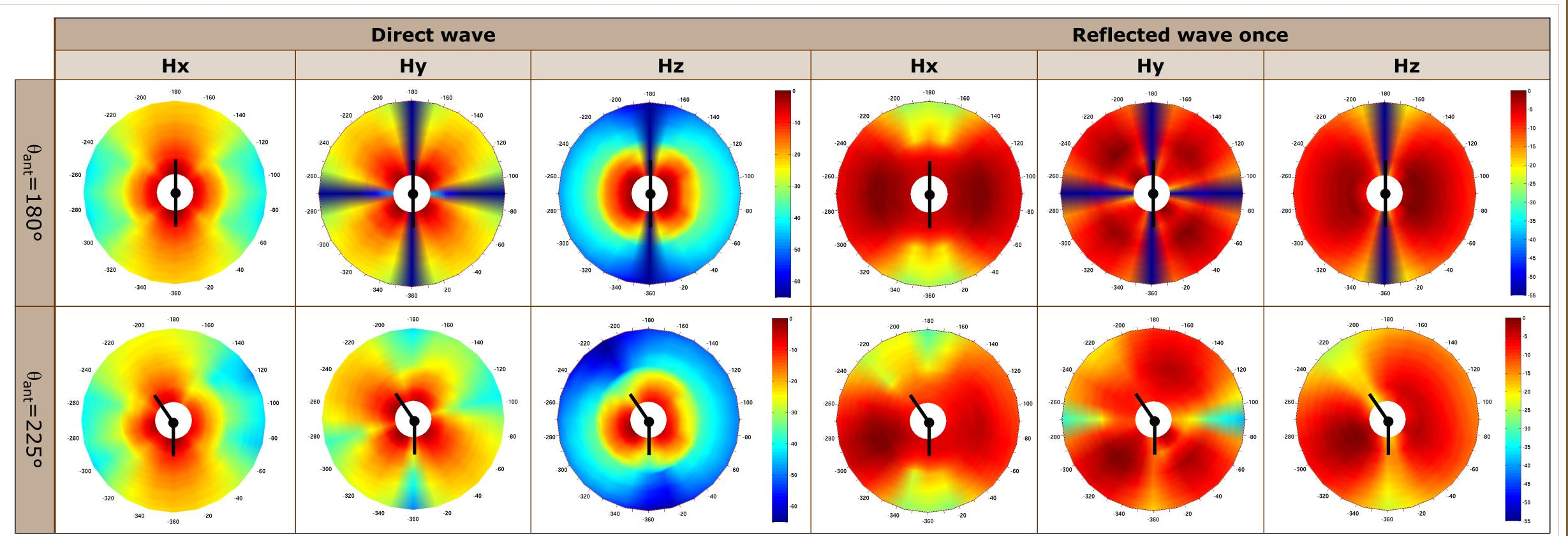
Amplitude map of the three magnetic field components of the direct wave and the reflected wave, for a distance Lander-Rover ranging from 100 to 500m. The configuration with two monopoles perfectly aligned  $=180^{\circ}$  is also shown for a reference.
